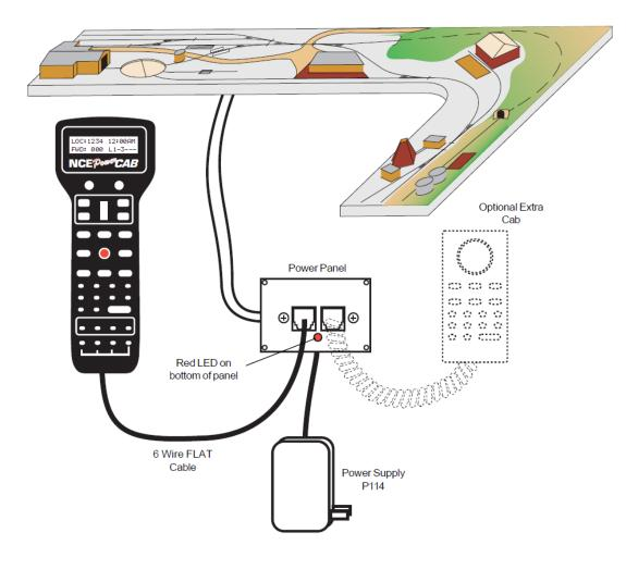
Command Station & Throttle (Cab) Power Supply Power Panel
