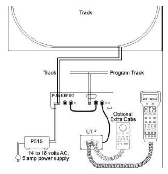
Command Station Throttle (Cab) Power Supply Power Panel + Booster Additional Cabs
